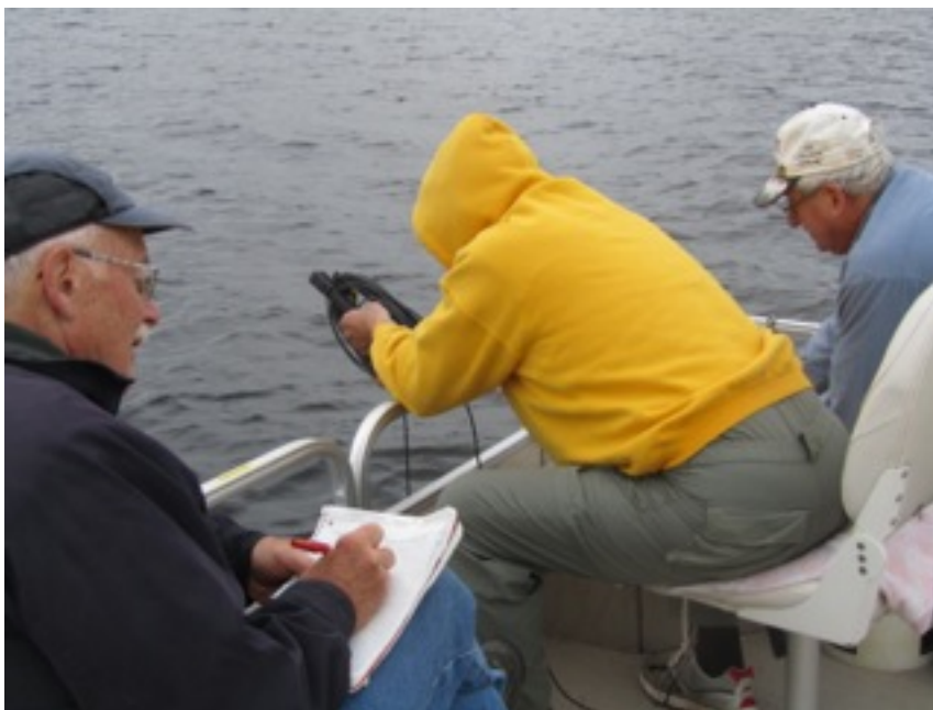
Ed, Frosty, and Larry are using a dissolved oxygen meter to compile temperature and dissolved oxygen concentrations. They observed the thermocline starting at about 16 feet.
