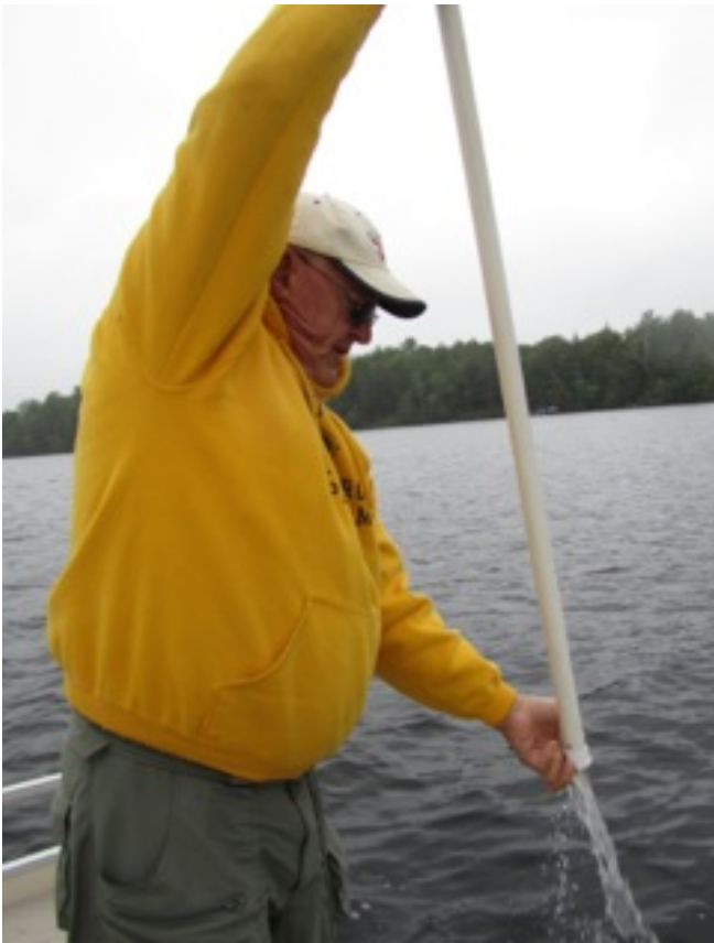
Frosty is testing the lake sampler tube used to collect a water sample at the 3-6 foot depth.
