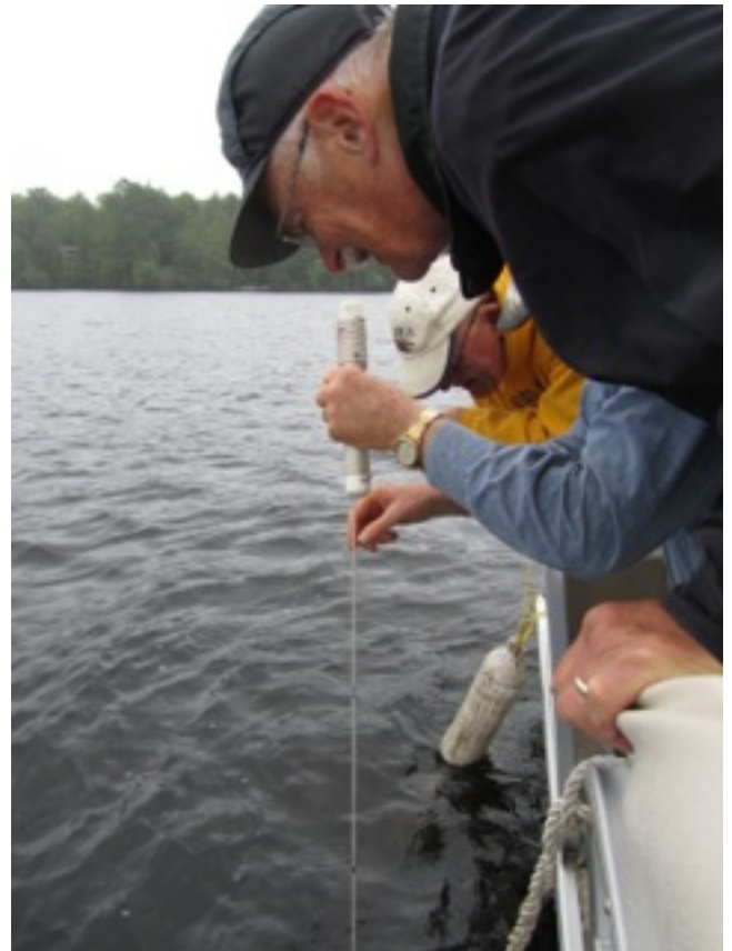
Diamond Lakers take a water clarity reading defined as the depth where the black and white secchi disk attached to the measuring cord disappears from view.
